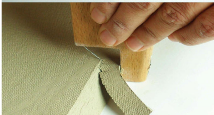
X-BEVEL-10108 Bevel cutter with 30, 45, and 60 degree cutting wire
